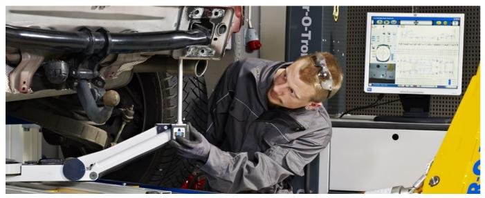
Through sensors in each joint and a measuring head underneath, the measuring slide communicates wirelessly with Vision2, delivering real-time measuring data three times per second. The built-in, versatile remote control lets the operator almost effortlessly manage the entire measuring process without having to be at the computer.
