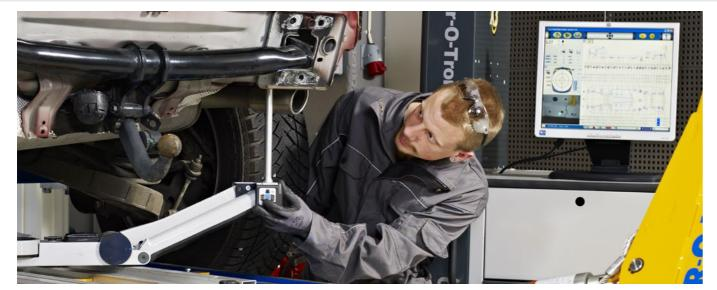
Through sensors in each joint and a measuring head underneath, the measuring slide communicates wirelessly with Vision2, delivering real-time measuring data three times per second.
