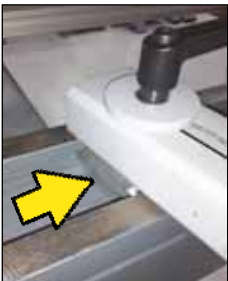
The holding arm cam lock tightened in 90° angle to the bench tracks.
