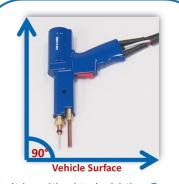
It is critical to hold the Gun vertically straight at a 90° Angle to the surface of the vehicle to ensure that the 2 mm gap is maintained when the grounding rod is adjusted.
