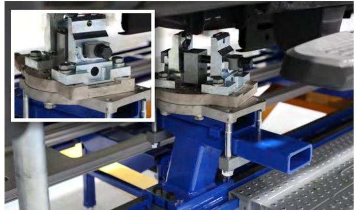
Clamps rotate to accommodate new angled frame designs
